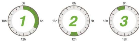
With 3 definable periods, users can freely set the mains charge/loading period in the range of 00:00–23:59. During the period set by the user, in case of PV energy output, it will be used first; in case of no PV energy output or lack of PV energy, mains will be used as a supplement.
