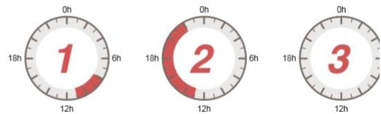
With 3 definable periods, users can freely set the battery discharge period in the range of 00:00–23:59. During the period set by the user, the inverter will first use the battery inverter to load; if the battery power is insufficient, the inverter will automatically switch to mains to ensure stable operation of the load.
