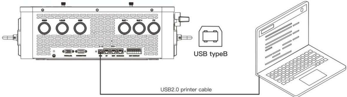
Users can use the upper computer software through the port to read and modify device parameters. If needing the installation package for the upper computer software, you can download it from the official website of SRNE, or contact us to get it.
