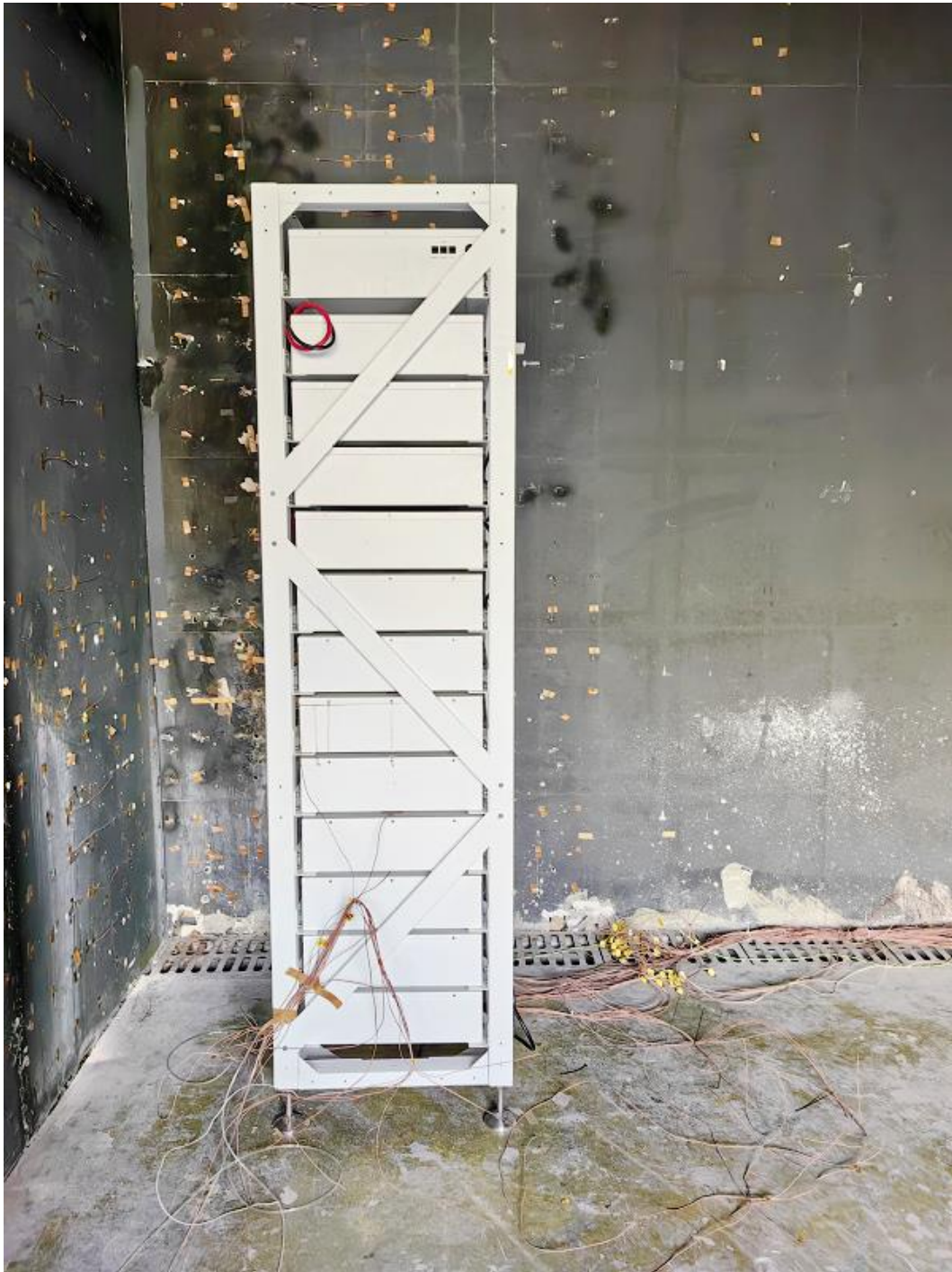
Figure 17. Photo 01 of initiating BESS unit after test.
