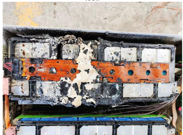
Figure 21d. Photo 02 of thermal runaway location.
