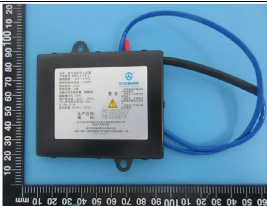
Figure 3f View of Aerosol unit (Internal side of battery pack)
