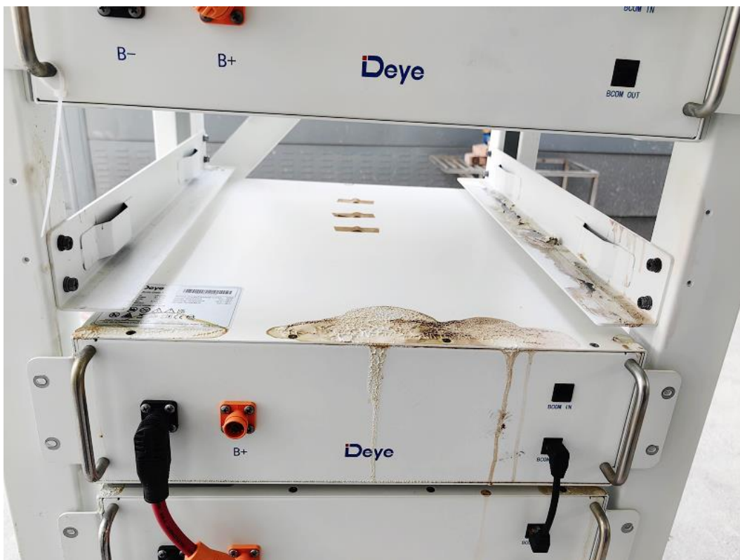
Figure 20. Photo 04 of initiating BESS unit after test.
